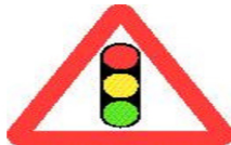
Traffic signals ahead
